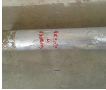
Fig: 2.1.2 Glass fibers with Epoxy resin in Al tube
