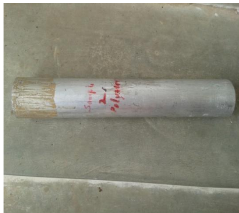
Fig: 2.1.1 Glass fibers with polyester resin in Aluminum tube
