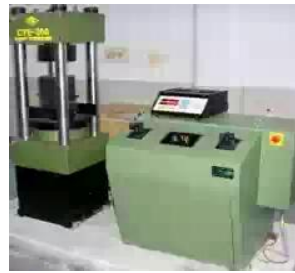
Fig: 3.1 UTM used for compression testing of columns
